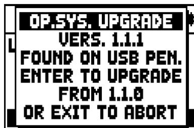
In this phase the system checks the upgrade installation files in your flash drive. As written on the pop-up, press [ENTER] to proceed, or [EXIT] to abort.
